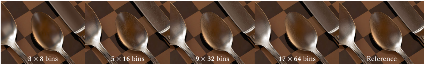
Fig. 15. We rely on a spherical histogram that discretizes the upper hemisphere into bins (see Section 4.1). The resolution of this histogram directly impacts the minimally reproducible detail size: lower resolutions progressively lose detail in the normal map, effectively smoothing it out. Our selected setting ( 9 \times 32 ) is adequate for all scenes we have tested, when compared to the ground truth.
