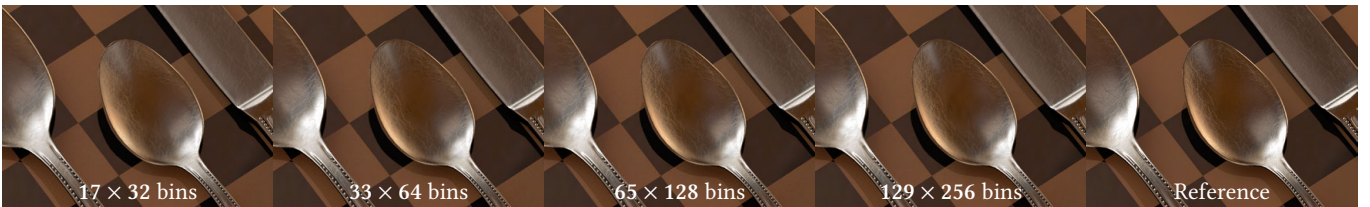
Fig. 16. Impact of the resolution of the rotated ZH Gaussian roughness lobes (see Section 6.2). As is apparent, the resolution does not have a significant effect on image quality for the resolutions we tested. We use a conservative setting of 65 \times 128 .
