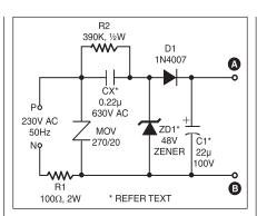
Fig. 1: The circuit of ultra-bright white LED lamp
