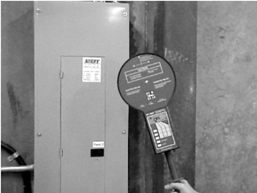
FIGURE 7.8 Low-frequency electromagnetic field meter used to measure magnetic and electric fields.
