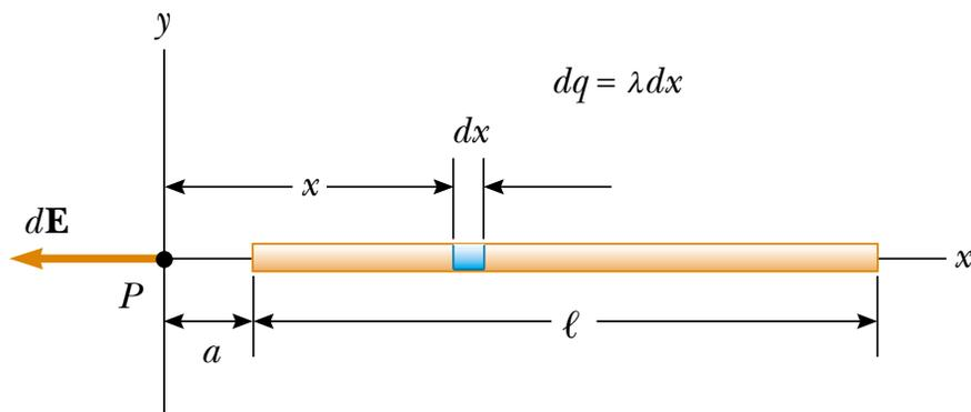
$$E = \int_a^{l+a} k_e \frac{\lambda}{x^2} dx \quad \text{ec. (2.11)}$$
